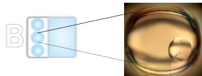
Figure 4: A schematic diagram of an Intelli-Plate well with 3 shelf positions and 1 reservoir (Art Robbins Industries, Sunnyvale, CA) and a cluster of protein crystals grown from an Echo liquid handler transfer (photo courtesy of Seth Harris, Genentech, South San Francisco, CA).
