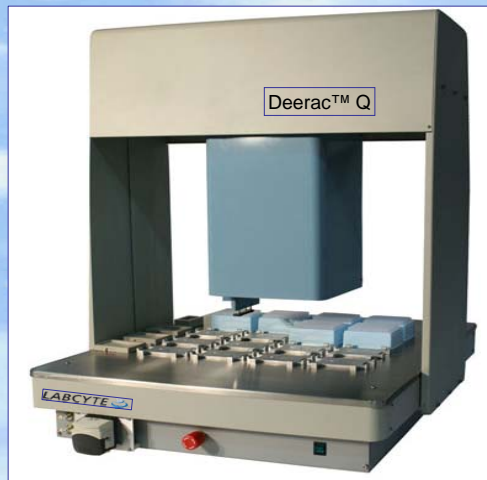
Figure 2. Deerac Q system. The Deerac Q deck and overhead gantry with the dual pipetting heads are shown. The deck has 16 plate positions which can be used for any combination of SBS standard plates, tip racks and waste. There are also four (4) reservoir positions for the Deerac MFC dispensing.
