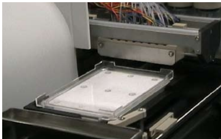
Figure 3. Filling a MicroClime lid with FlexDrop Dispenser.
