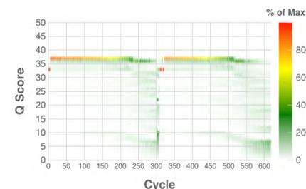
FIGURE 4: MiSeq sequencing statistics for 16S rRNA amplicon sequencing. Shown above is the Q-Score per cycle. The 16S rRNA amplicon sequencing is extremely low diversity, and 10% PhiX was spiked in to achieve these metrics.
