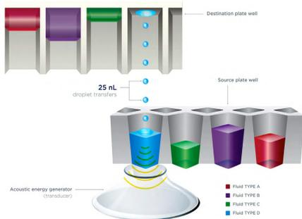
FIGURE 1: The Echo 525 Liquid Handler has a transducer that emits low energy sound waves to eject 25 nL droplets from a source plate to an inverted destination plate above.
